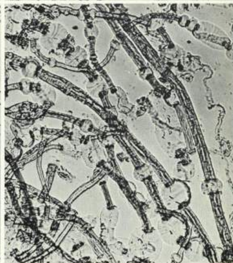
Plate 206. Daphne papyracea paper fibres. Notice the stronger staining of the paper fibres, the swelling, the indistinct fibre walls, the many flattened places and the dislocations, all due to the chemical and mechanical treatment of the paper fibres. To the left a long pointed sclereid fibre. Magnification \times 240 .
