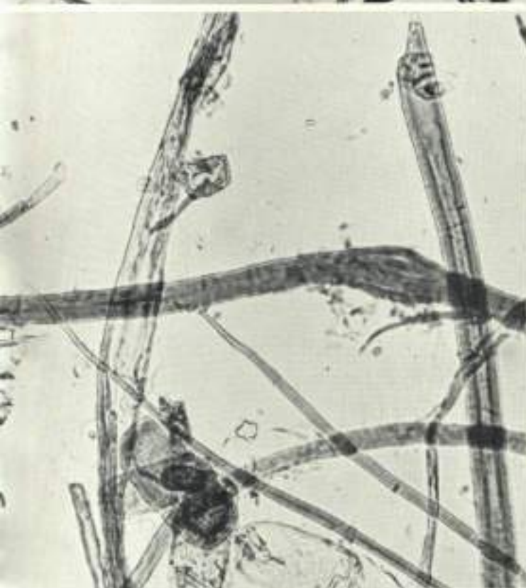
Plate 236. Fibres from handmade paper made of rice straw fibres at the small factory in Tripureswar, Kathmandu. Notice the long, thin, pointed fibres and also the indented epidermis cells. Magnification \times 240 .
