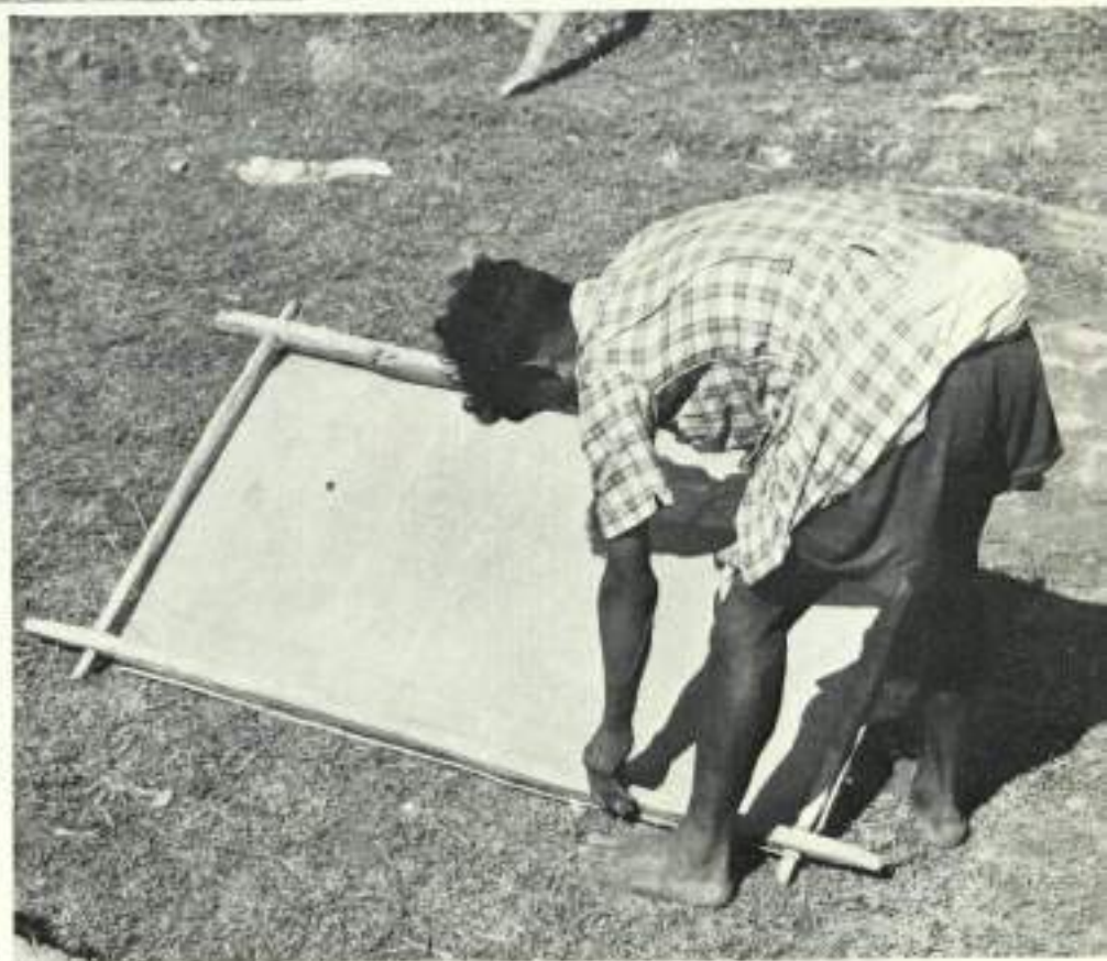
Plate 93. The wet mould is dried by leaning it against a stick and letting it dry in the sun and wind.
