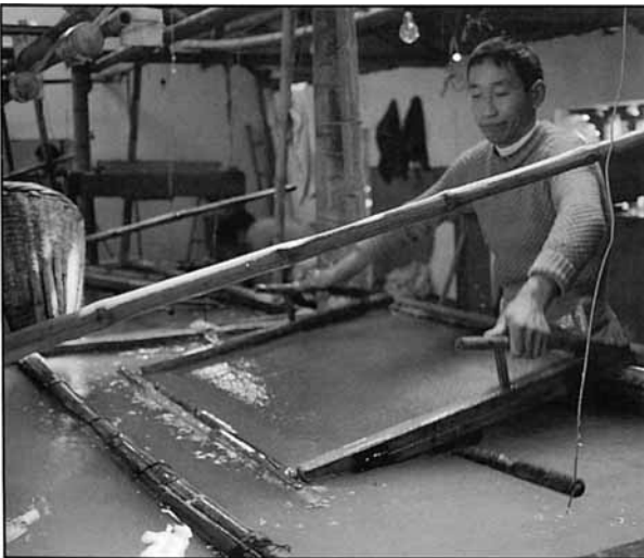
Fig. 4 A paper factory in Zhejiang province. The papermaker is forming a sheet on a bamboo screen.
