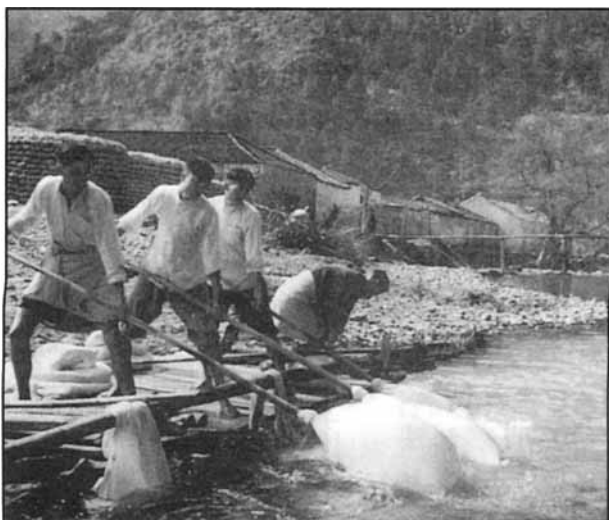
Fig. 6 Fine mesh bags of rice pulp are suspended in fast flowing water to remove impurities and bleach.
