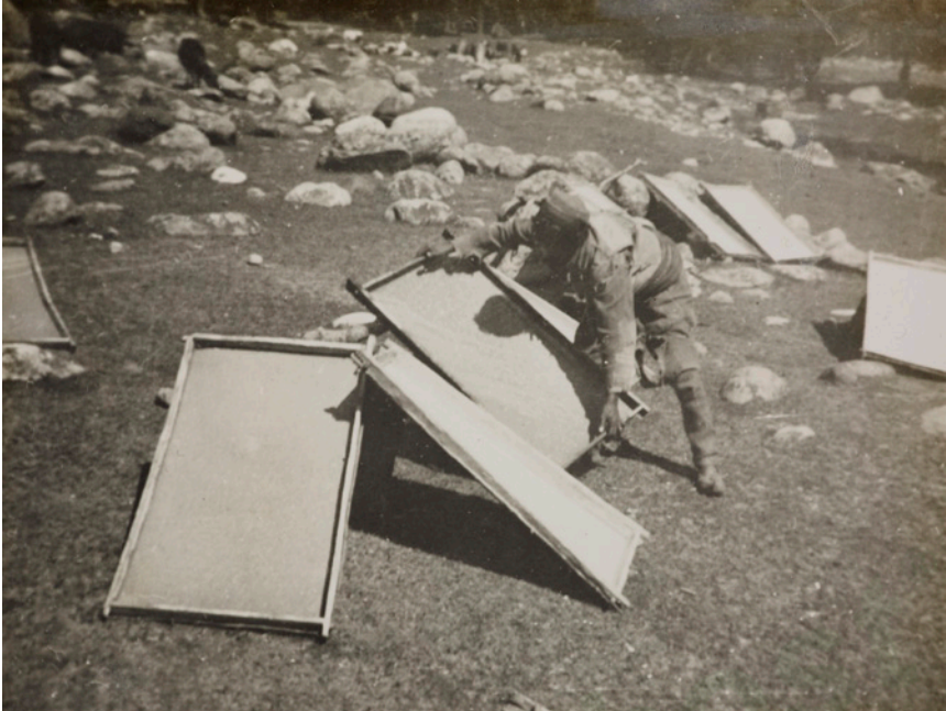
FIGURE 115 Drying process during papermaking in the Kullu Valley, Himachal Pradesh, 1940s. The papermaking molds with newly made sheets of paper are left until the sheets are dry. Photo 523/1(154), © The British Library.
