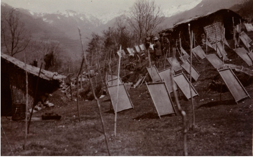
FIGURE 112 Drying process during papermaking in the Kullu Valley, Himachal Pradesh, 1940s. The papermaking molds with newly made sheets of paper are left until the sheets are dry. Photo 523/1(154), © The British Library.
