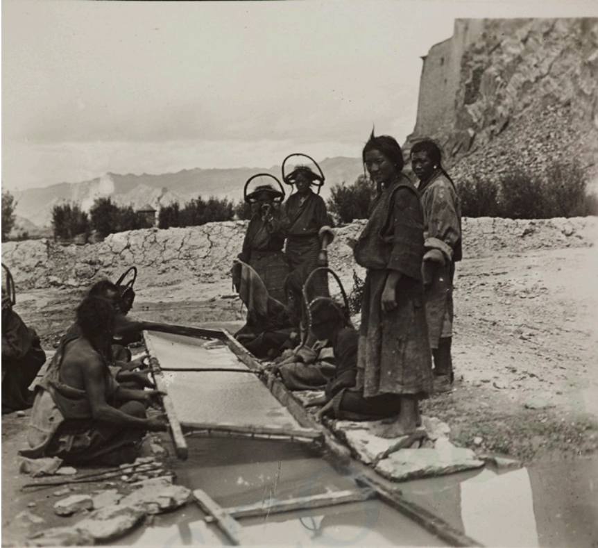
FIGURE 116 A large size 'floating' mold, constructed with a wooden frame and attached woven textile, placed in water (a stream) in Gyantse, c.1910–1920. Photo 112/2 (139), © The British Library.
