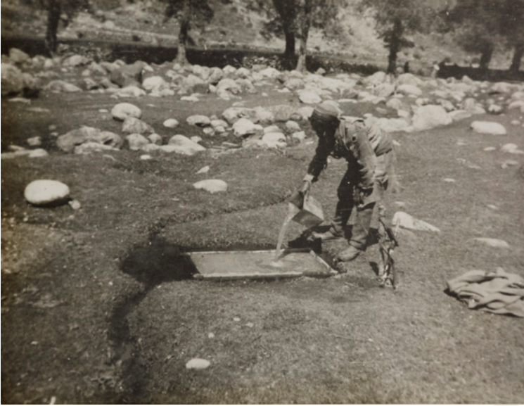
FIGURE 113 The process of making paper in the Kullu Valley, Himachal Pradesh, 1940s. Paper pulp prepared by beating upon a stone with a wooden mallet is being poured onto a 'floating' type of mold on the surface of a puddle. Photo 523/1(151), © The British Library.
